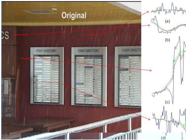
**Fig. 1.** Intensity profiles along the horizontal indicated by the red line. (a) Blurred rain streaks; (b) The edges with low pixel values; (c) The edges of different adjacency pixel values; (d) The clear background edges like rain. Blue line is pixel values of input image in a partial row to the same scale. The red line is the corresponding low frequency part via guided filter. The green line is the edge enhancement of red line.
