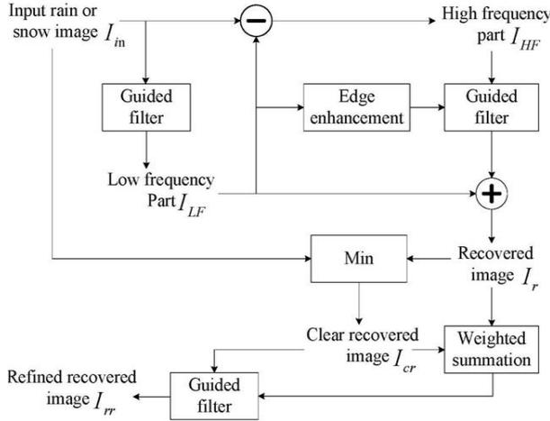
**Fig. 2.** Block diagram of the proposed removal method
